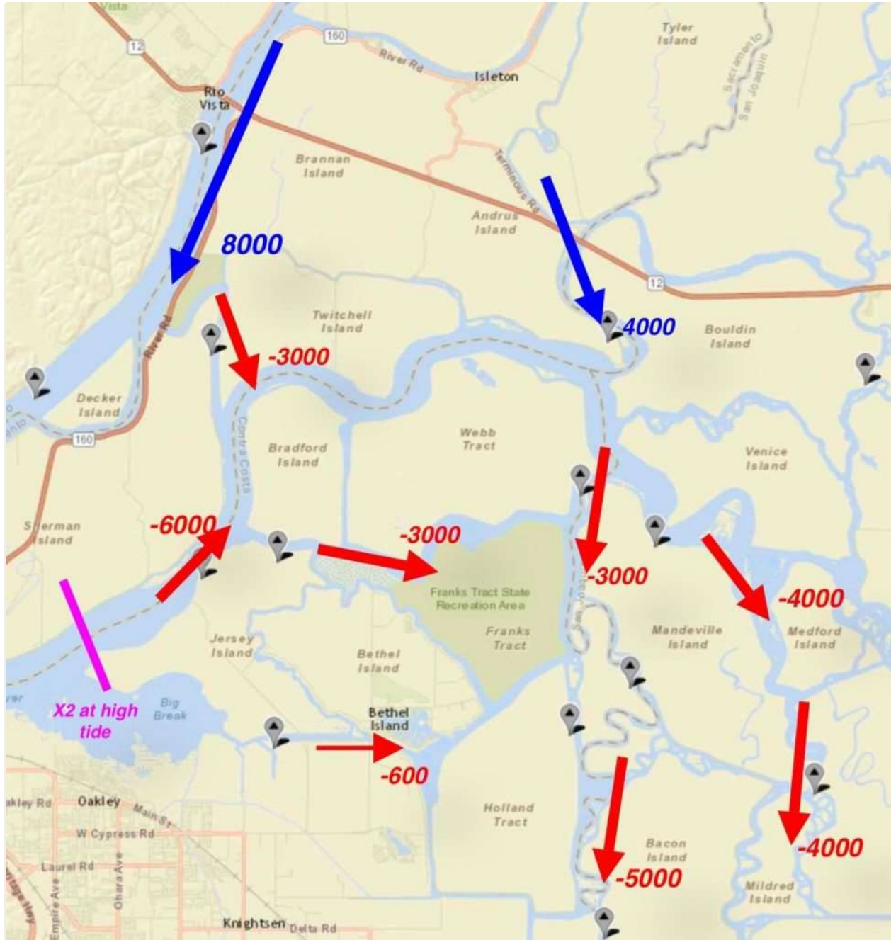
Figure 2. Net Delta hydrology (flow in cfs) on August 25/26 during a spring tide. Net Delta outflow is near zero with positive net flow in the Sacramento channel (north) and negative net flows in the San Joaquin channel (south). Exports were near maximum at 11,200 cfs. The location of X2 (2 ppt salt) at high tide is shown as magenta line.
